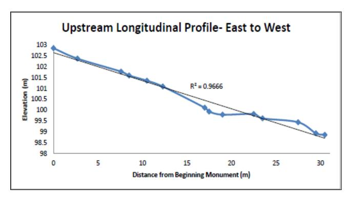
Figure 5: Upstream Longitudinal Profile
