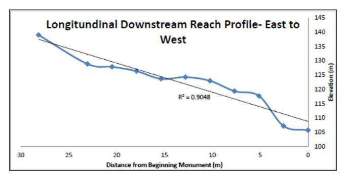
Figure 6: Downstream Longitudinal Profile
