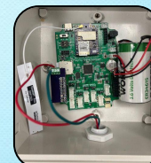
Mayfly Data Logger with LTE module
