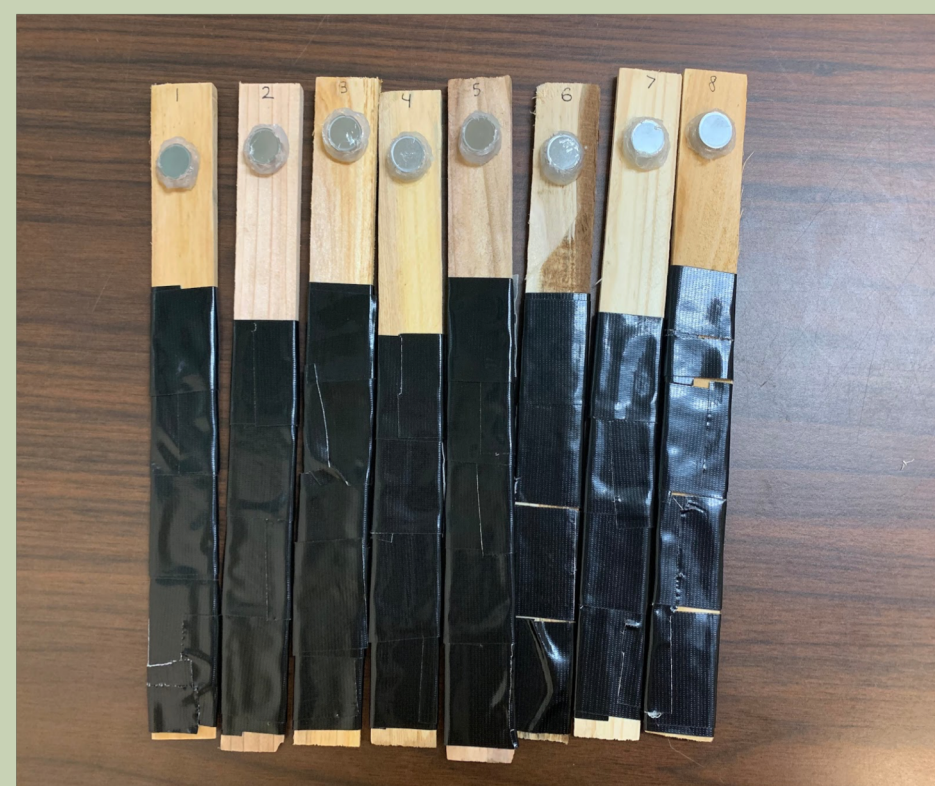
iButton sensors glued onto paint sticks with silicone sealant and reinforced with duct tape
